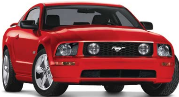
The "mag" wheels on the retro-styled Mustang are not magnesium, or even aluminum, but rather are Hayes Lemmerz spoked steel wheels clad in chromed plastic to create the appearance of vintage mags at an affordable price.
